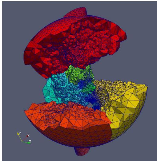
Domain/graph partitioning of unstructured mesh for 16 processors
